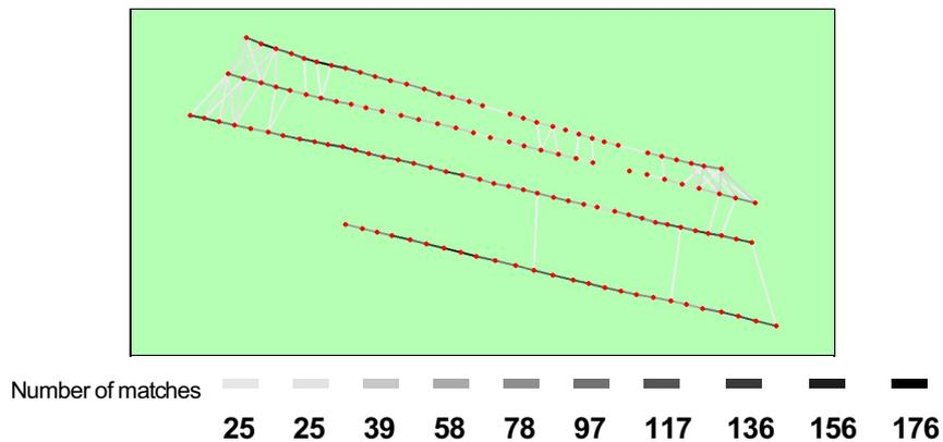
Figure 5: Top view of the geotags with a link between matching images. The darkness of the links indicates the number of matched 2D keypoints between the images. Bright links indicate low confidence and would require more overlap between the images or better quality images.
