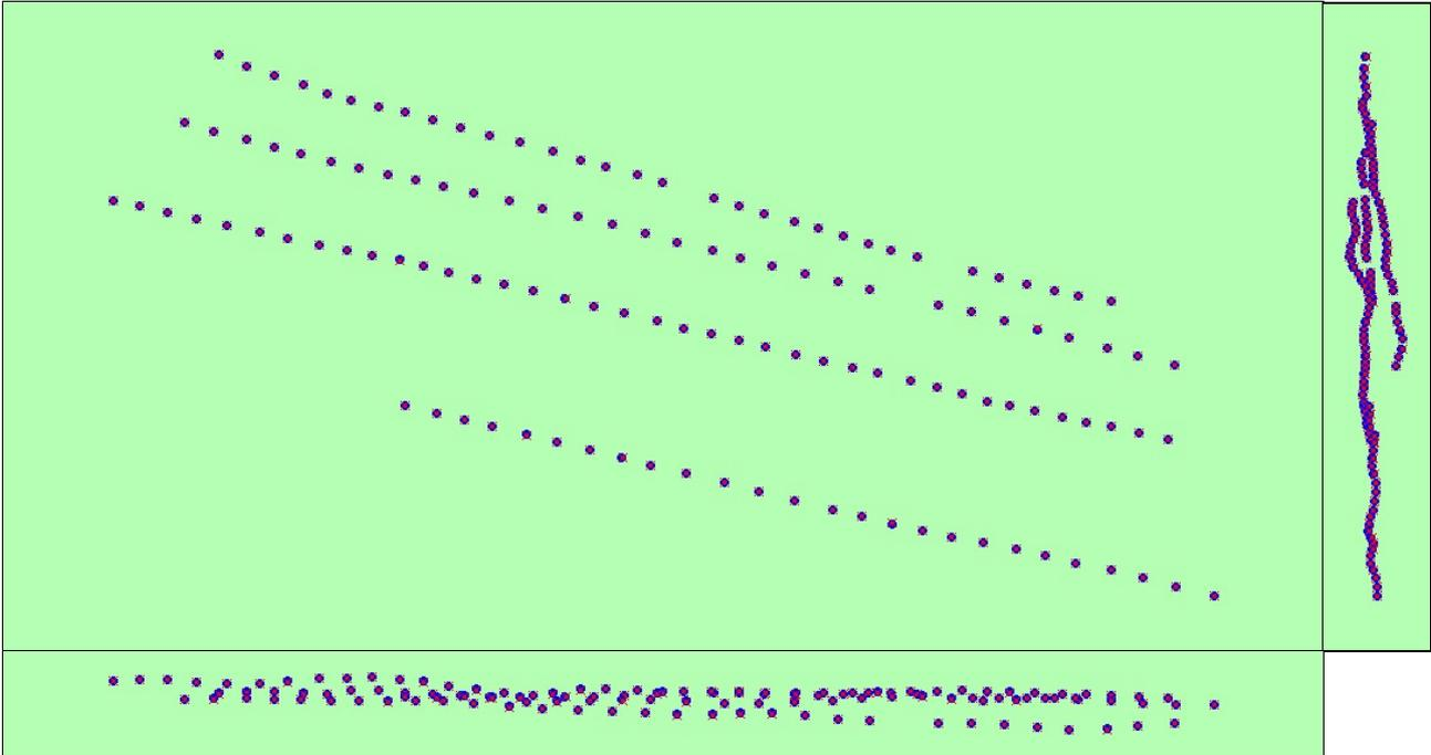
Figure 3: Offset between image geotags (small red crosses) and optimized positions (small blue dots) as well as the offset between the GCPs (large red crosses) and their optimized positions (large green dots) in the top-view (XY plane), front-view (XZ plane) and side-view (YZ plane).
