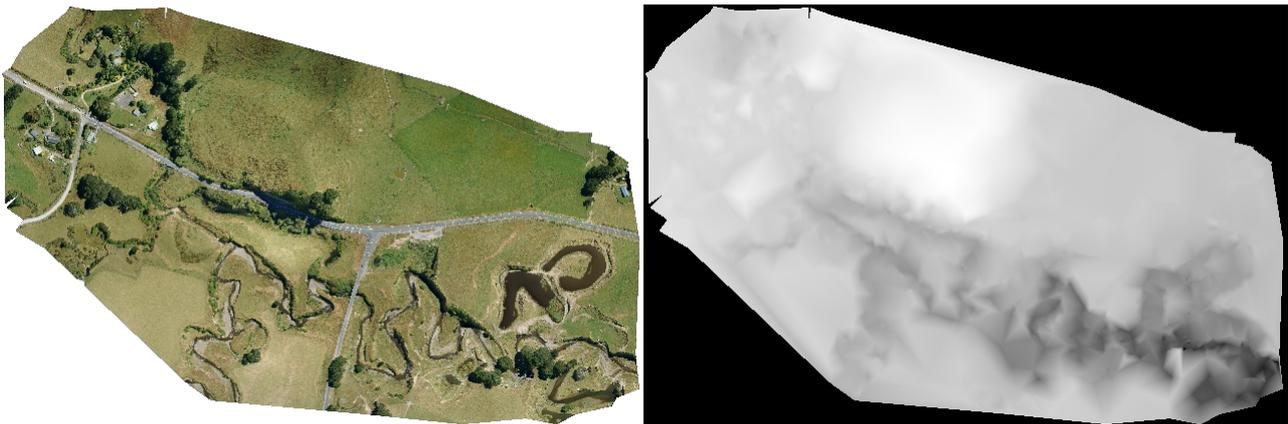
Figure 1: Ortho mosaic and the corresponding sparse digital elevation model (DEM) before densification.
